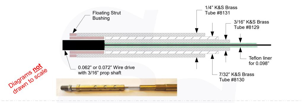
Stuffing Tube and Wire Drive Assembly Option #2 With Strut Bushing and Larger Diameter Teflon Liner
